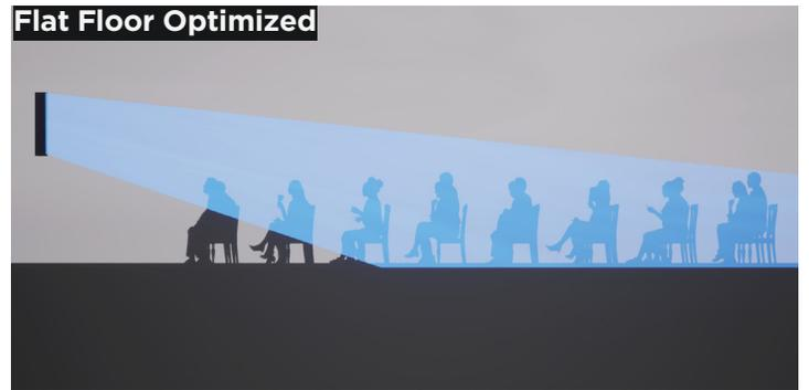
Flat floor optimized is ideal for flat floor seating with the array bottom mounted slightly above ear height of audience. It provides consistent coverage from the front to the back row.
