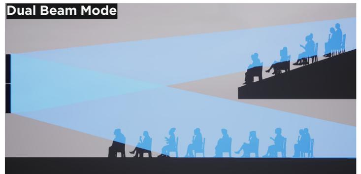
By utilizing all the drivers of the array for both beams simultaneously, Dual-beam mode allows you to use any two beam patterns independently.
